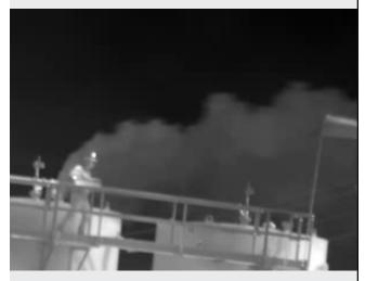
Oil and gas industry worker on tank catwalk and inside gas leak from open thief hatch.
