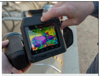
Images and videos from OGI devices such as the FLIR GF77 can provide a fact-base for troubleshooting safety and operations issues.
